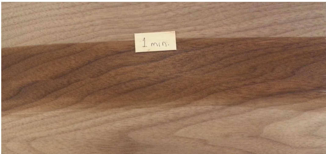
After 1 minute of sanding and wiped with mineral spirits. No glue was observed
