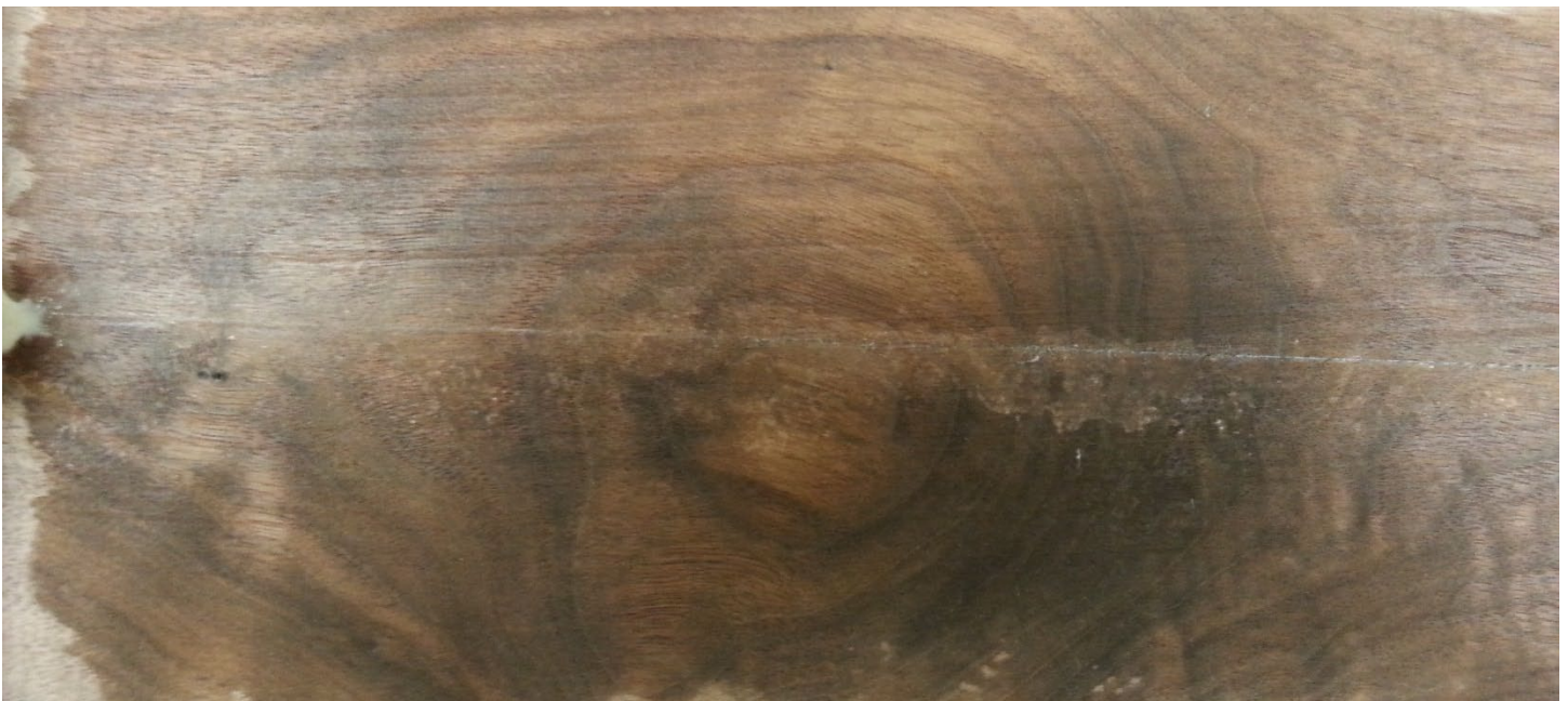
A slow wiping process (16 minutes). 18 rolls of the cloth and then some of the glue dried on the surface. Wood is water soaked and the grain is raised.
