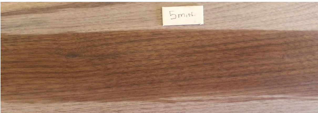
After 5 minutes of sanding and wiped with mineral spirits. No glue was observed.
