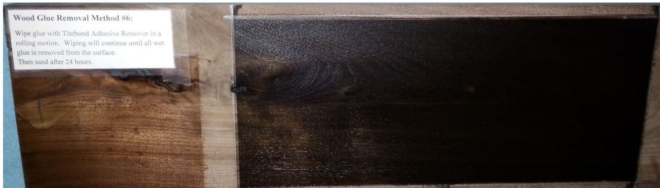
Stained and finished glue joint. No glue was observed.
