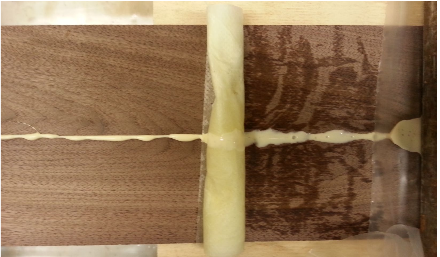
Wiped the glue with Titebond Adhesive Remover in a rolling motion.
