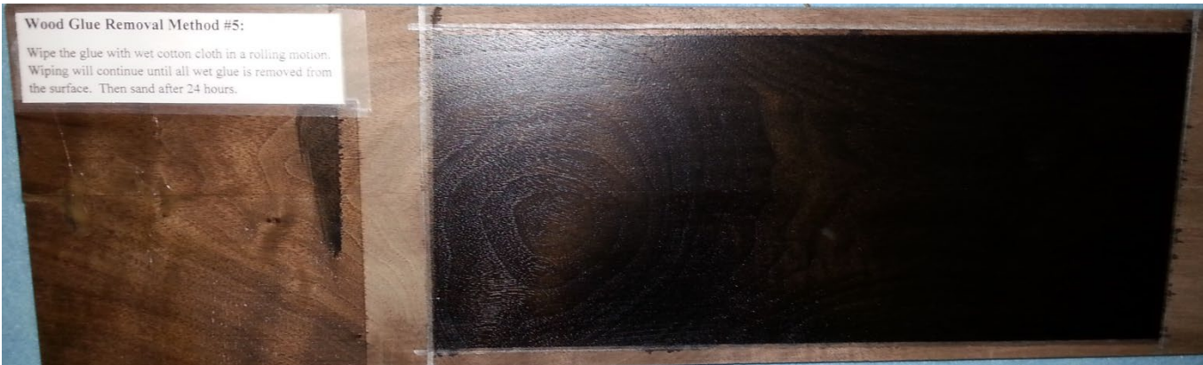
Stained and finished glue joint. No glue was observed.
