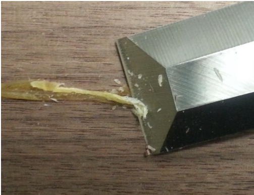
Scraping off excess glue with a sharp chisel.
