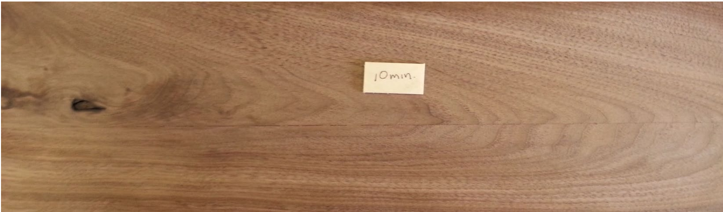
After 10 minutes of sanding. Oil from the wipes that was left on the surface of the wood was removed after the removal of the glue.
