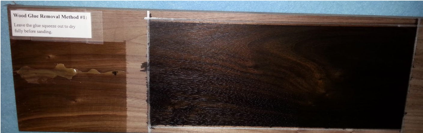
Stained and finished glue joint. No glue was observed.
