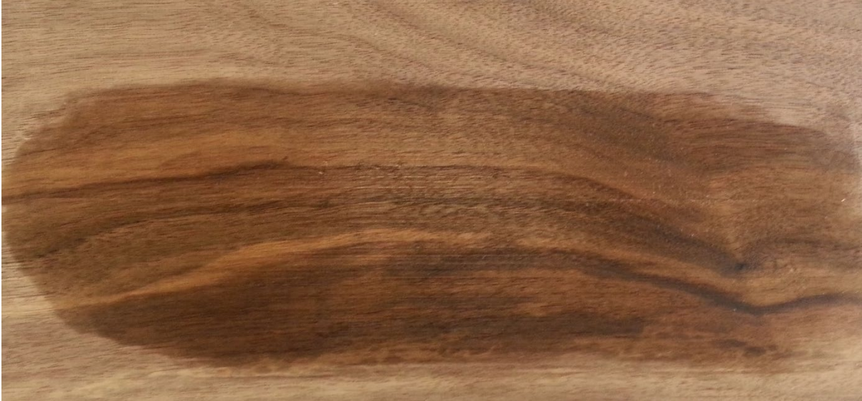
After the water was dried, and then wiped with mineral spirits. No glue was observed.
