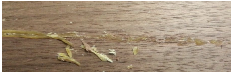
The glue did not peel off but came off in chunks and pulled off wood fibers.
