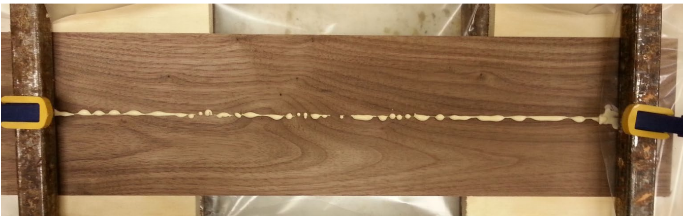
Clamping @ 200psi and achieving glue squeeze out, creating a joint.
