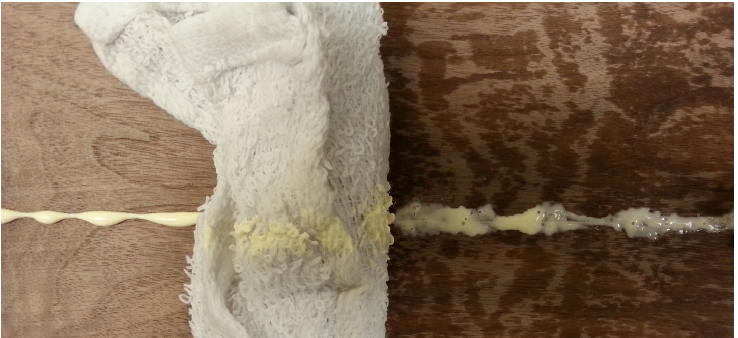
Wipe the glue with a wet cotton cloth in a rolling motion.
