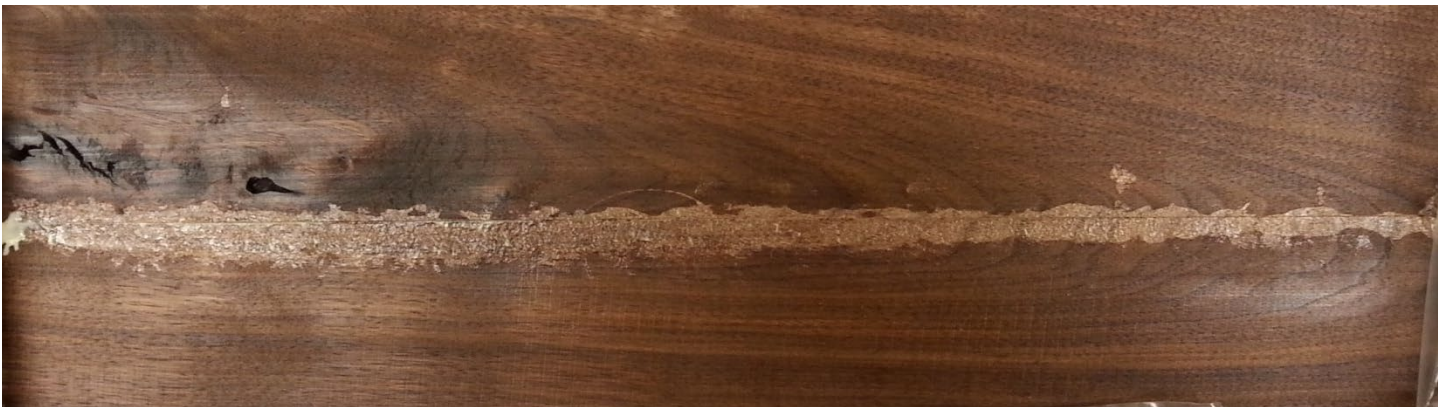
A very slow wiping process (20 minutes). 16 rolls of the cloth and then some of the glue dried on the surface. Oil from the wipes was left on the surface of the wood.
