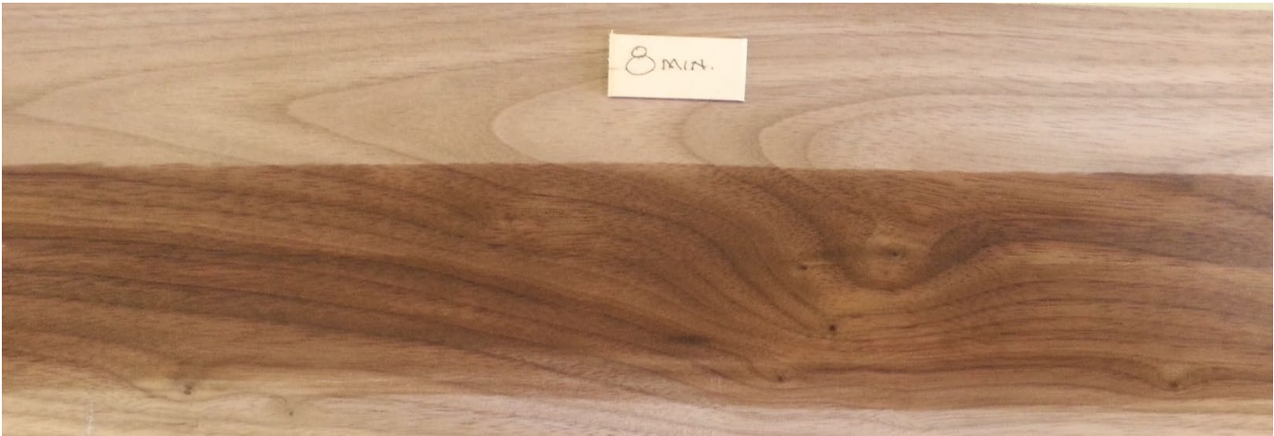
After 8 minutes of sanding and wiped with mineral spirits. No glue was observed.
