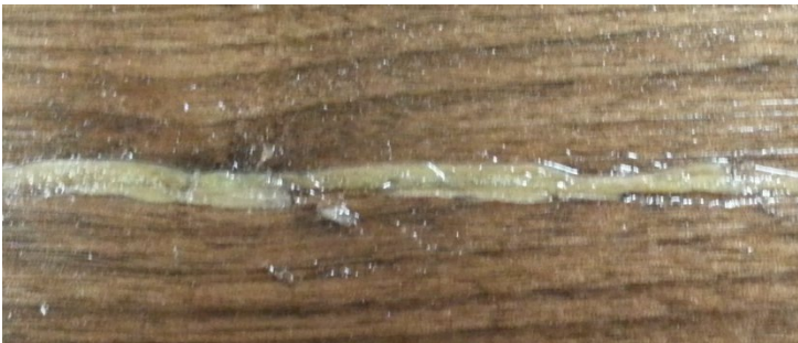
Wiped with mineral spirits showing dried glue.
