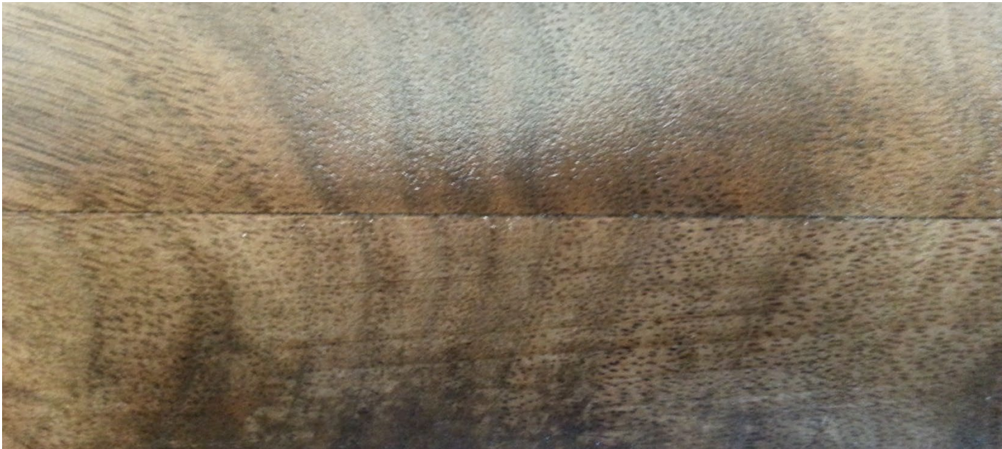
Wiped with mineral spirits. No glue was observed
